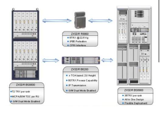
The Wireless Lab, to be built, will include mainly the most cutting-edge solutions for next generation mobile network, such as ZTE SDR solution, which can combine **GSM and WCDMA** network together.
